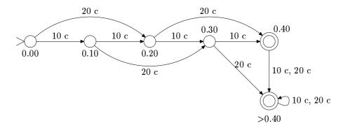
Formally, a deterministic state machine (finite automaton) is a tuple  $M = (Q, \Sigma, \delta, q_0, F)$ , where Q is finite set of states,  $\Sigma$  finite alphabet,  $\delta$  function  $Q \times \Sigma \to Q$ ,  $q_0 \in K$  initial state and  $F \subseteq Q$  set of accepting states.
