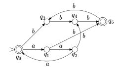
b) Language  $L = \{w \in \{a, b\}^* \mid w \text{ contains as many } a \text{ and } b \text{ letters modulo } 3\}$  is recognized by the following finite automaton:
