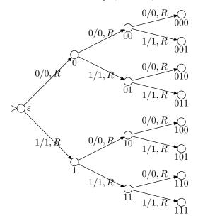
If the machine ends in the state 011, then the input symbol is  $a_3$  since  $011_2 = 3_{10}$ . The symbol that is written to the tape is similarly done using k different transitions. Finally, the tape head is moved k steps to the correct direction.
